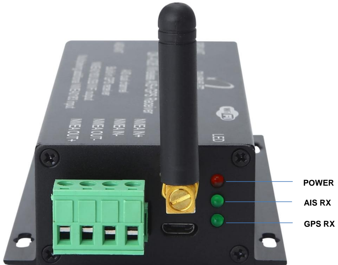
Figure 3 USB and NMEA input/output connector
