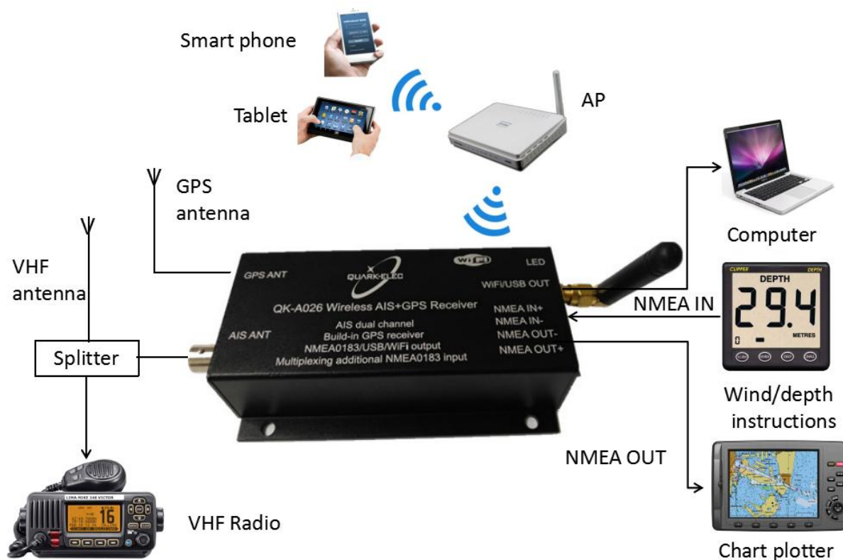
Figure 9 Station Mode Connection
