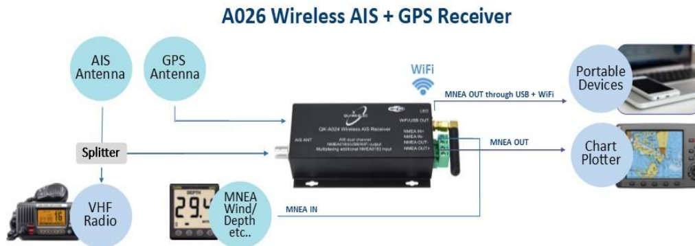
Figure 1 QK-A024/26 Connection Diagram
